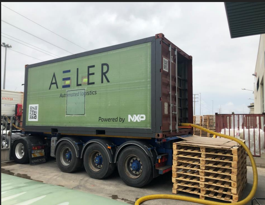
The AELER composite container loaded with 28KL Trust flexitank
